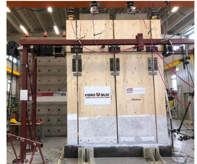
Full scale cyclic test
